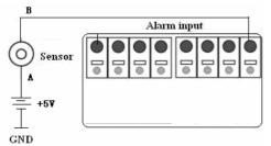
Fig 2.7 Sensor Connection
